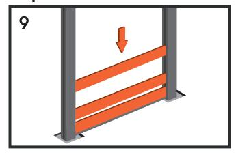
Slide the initial Fence Board down the post grooves and into the Bottom Trim. Once secure, slide the next Fence Board down the post grooves onto the previous Fence Board.
