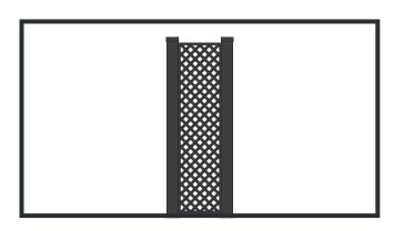
The Trellis can be used to create semi private spaces within your fencing. This is done by installing the Trellis between two posts in a vertical position.
