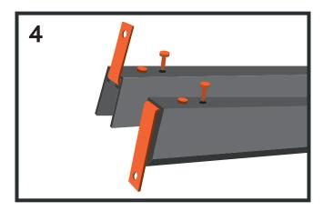
Fasten the bracket into the Top Trim with the provided screws and tighten with a crosshead (Phillips) screwdriver. Repeat with the Bottom Trim.
