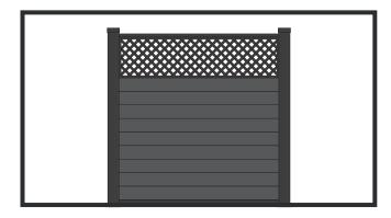
Secure the Top Trim to the Fence Post using the screws provided.
