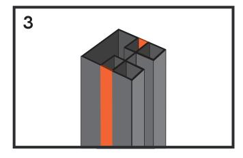
The Fence Posts can also be utilised in an 'L' shape and 'T' shape design by removing the relevant post slot closure piece.
