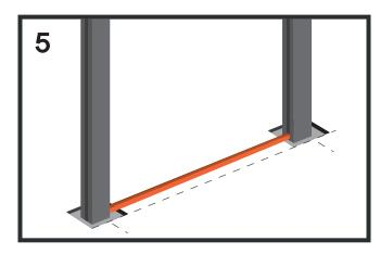
Using a string line, measure the distance to the next post. This should be done from centre to centre of the posts.
