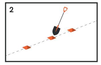
For most installations, a hole dug out to a recommended depth between 600–850mm is generally appropriate, depending on individual site and ground conditions. Remove any rocks or roots.
