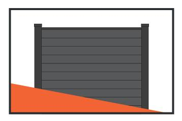
**Installation Top Tip** - If you are installing the fencing on a gradient or slope, mitre (cut) the respective Fence Boards to the desired angle and length.
