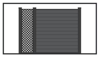
Cut the Top & Bottom Trim to the desired length, and fasten the brackets in place.
