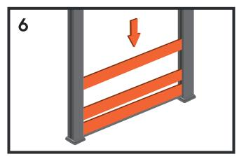
Slide the initial Fence Board down the post grooves and into the Bottom Rail Trim. Once secure, slide the next Fence Board down the post grooves onto the previous Fence Board.
