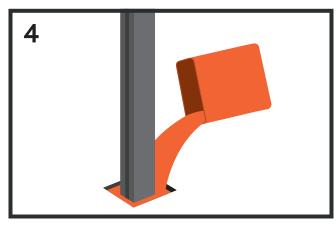
Fill the hole with a suitable cement based product, to suit ground conditions.
