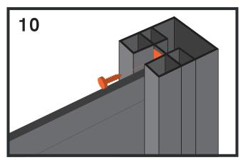
Secure the Top Trim to the Fence Post using the screws provided.
