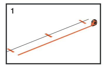
Mark out the line of the fence using a string line, ensuring that the area is free of any obstacles. Ensure that you install the posts on your side of the boundary.
