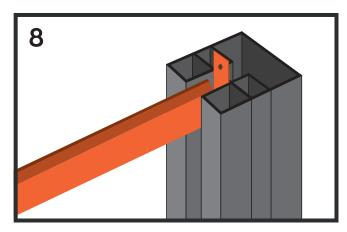
Insert the Bottom Trim into the grooves on the posts, aligning it at both ends.
